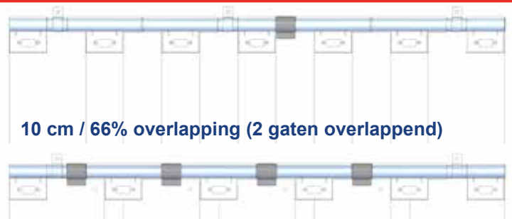
10 cm / 66% overlapping (2 gaten overlappend)
