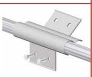
A Slide the overlapping strips over the bolts. Alternately assemble the strips concavely and convexly. For a 10cm overlap use both pre-punched holes and for a 5cm overlap only use the outer holes.
