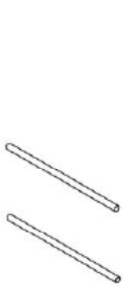
2 x pipe Ø25,4 x 1,0 mm L = 600 mm
